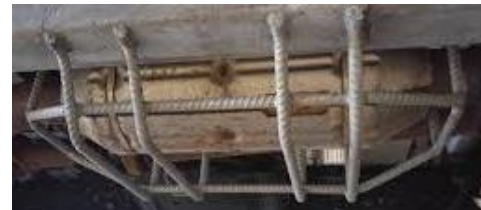
An example of a DIY Catalytic Converter Theft Prevention Cage
